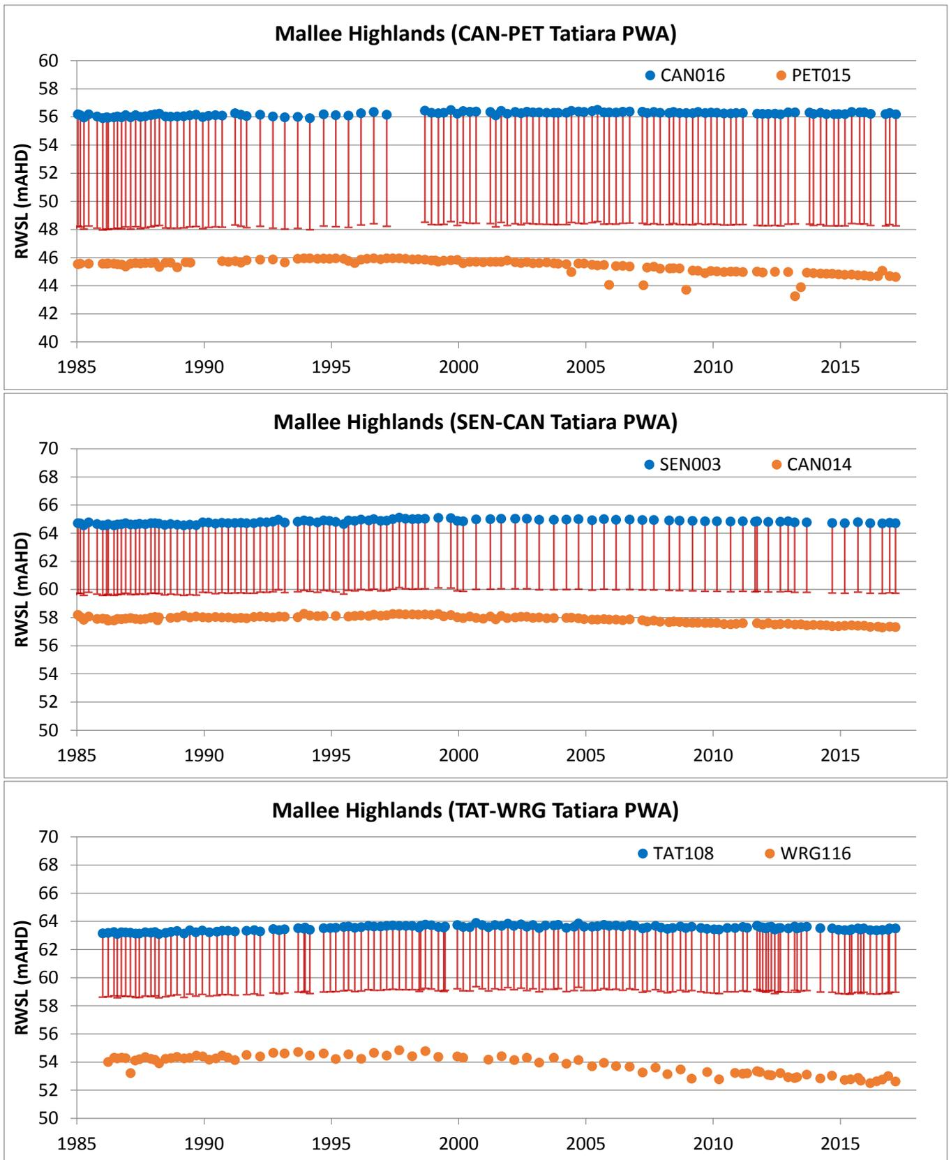
Figure 4.5. Western pairs of observation wells in the Mallee highlands noting that red error bars represent the difference in water level for which the 0.0004 RCL would be exceeded
