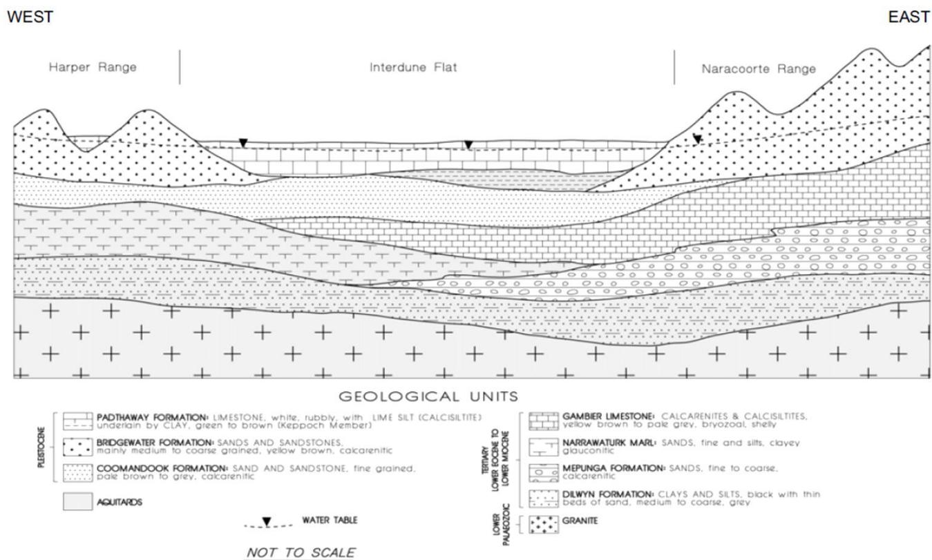
**Figure 2.2. Hydrogeological cross-section in the Padthaway PWA (Harrington et al., 2006)**
