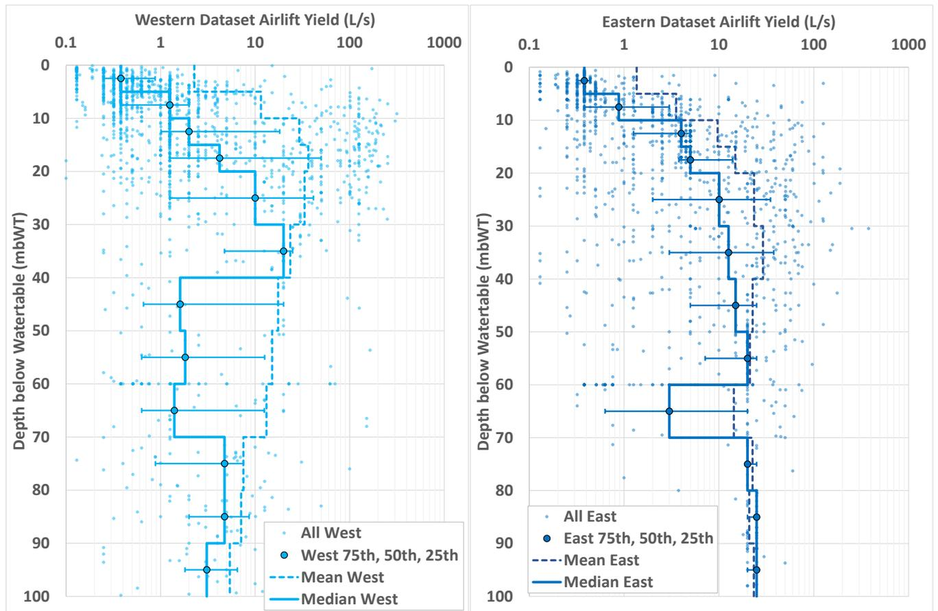
Figure 6.2. Plot of the airlift yield vs total well depth below watertable for the western and eastern datasets
