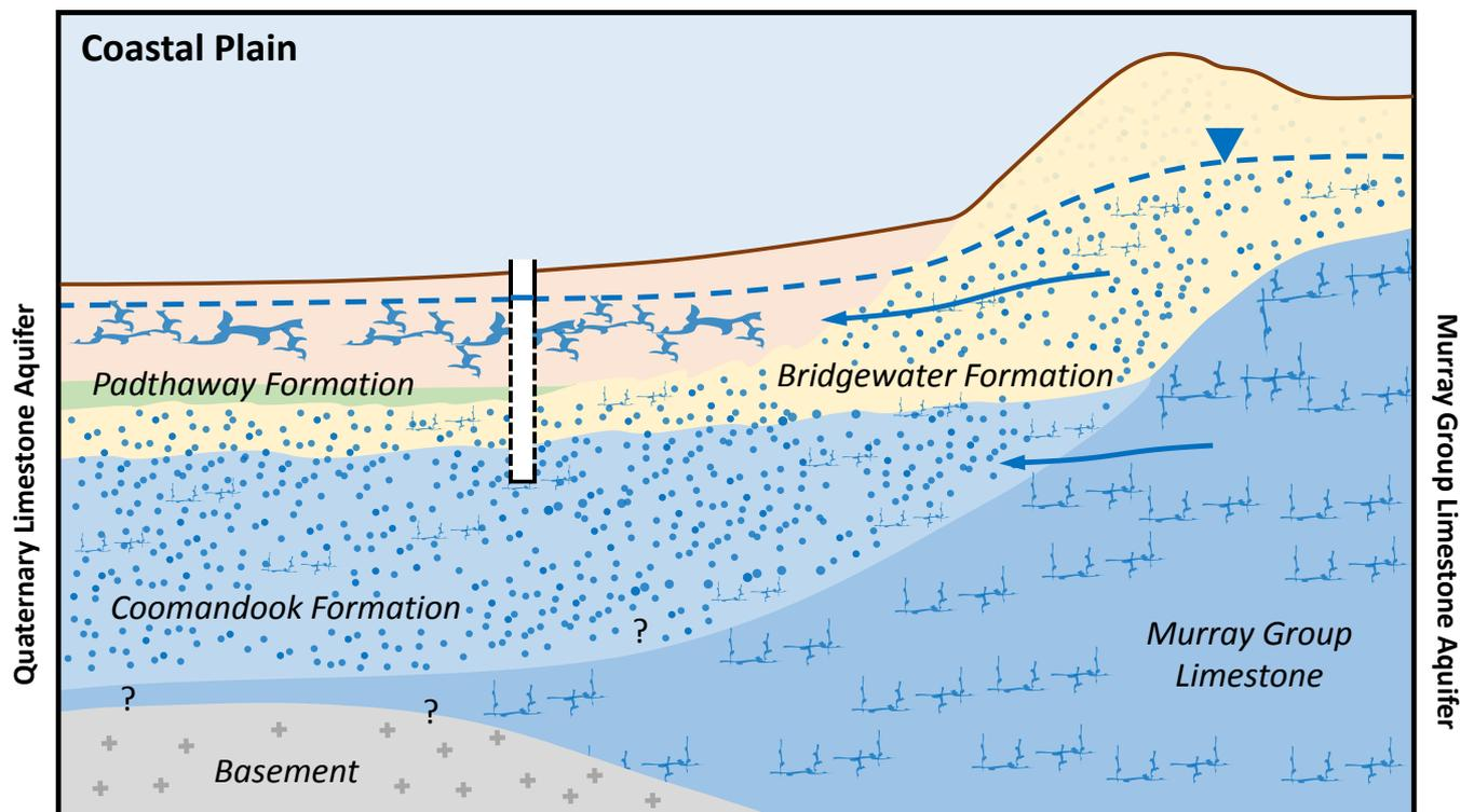
**Figure 2.9. Hydrogeological conceptual model of the Quaternary limestone aquifer in the coastal plain with groundwater salinity increasing to the west**
