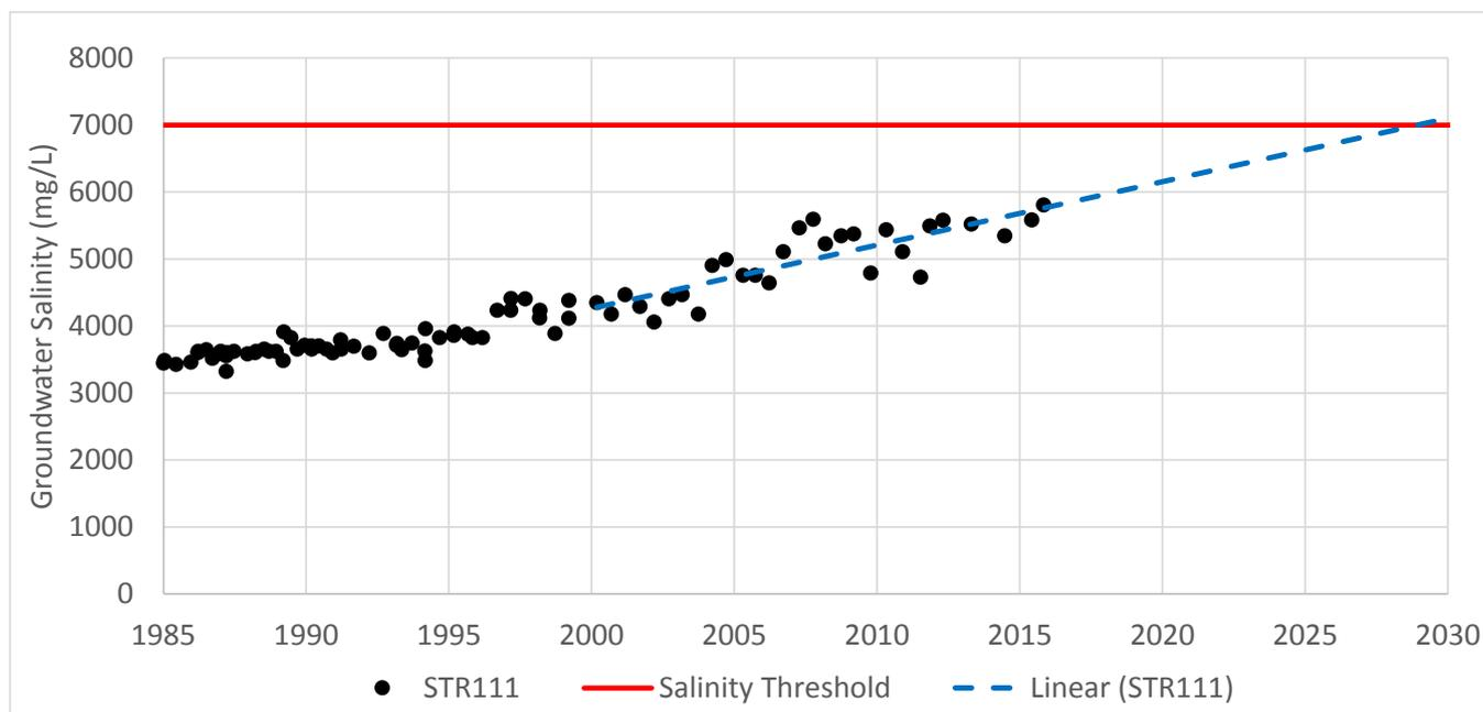
**Figure 3.1. Recent groundwater salinity trend (2000–present) trajectory for STR111 on the coastal plain**
