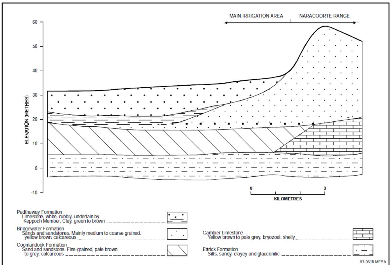
**Figure 2.1. Hydrogeological cross-section in the Padthaway PWA (Brown, 1998)**
