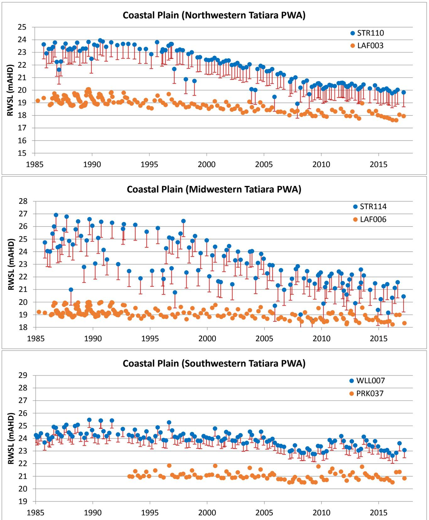
**Figure 4.2. Potential hydraulic gradient RCLs for coastal plain noting that red error bars represent the difference in water level for which the 0.0001 RCL would be exceeded**
